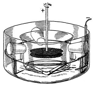
side of this was placed a beaker of smaller diameter, without a bottom and supported so that its lower edge extended just below the surface of the mercury. The inner cup was held in position by means of three
